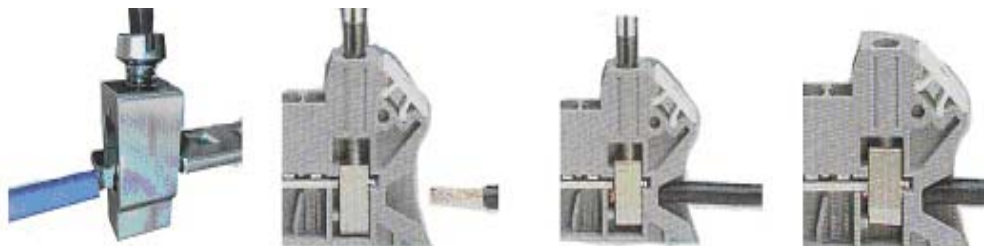
Figure 5-10 Sketch map of wiring method of wiring terminal
